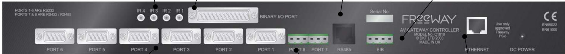
6 x RS-232 serial ports on 9-way male D-Type connectors. Used for controlling RS232 compatible equipment
